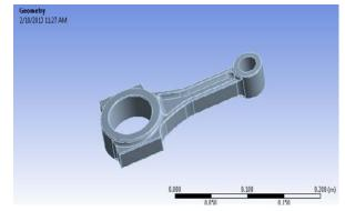
The procedure of using FEM usually consists of following steps. (a) Applying the material; (b) meshing; (c) determining and imposing loads and boundary conditions; (d) solving ; (e)simulation.
